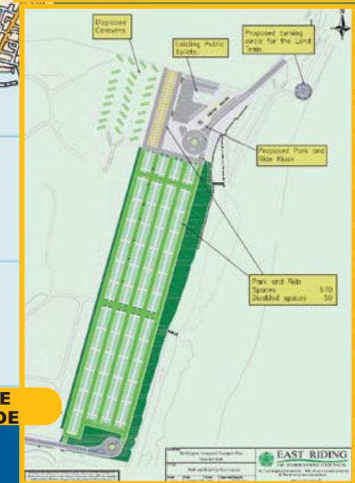
The main work is to provide a 1000 space Park and Ride facility on the existing South Cliff Car Park. A new access road will serve the facility from the A165 through the South Cliff Caravan Park. Displaced caravans will be mainly relocated to the existing boat compound with the remainder spread through the caravan park. A dedicated bus and land train service will provide the "ride" into the town along the foreshore every 10min
